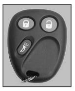
**Q** (Unlock): Pressing this button once will unlock the driver's door. The interior lamps will come on. Pressing unlock again within three seconds will cause the remaining doors to unlock.
